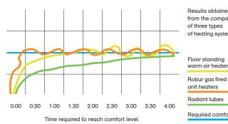
Results obtained from the comparison of three types of heating system
